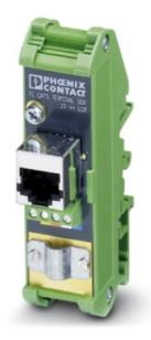
Passive connection field, 4 x screw terminal block on RJ45 female connector, pin assignment 1, 2, 3, 6, shield contacting to DIN rail, (mini patch field) as an alternative to on-site assembly with preassembled RJ45 patch cables
